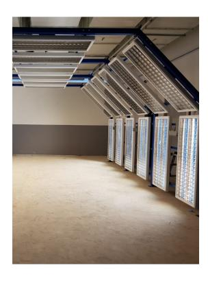
The light tunnels are also individualized and are customer-specific products that we design and produce based on the customer's needs. Our customers include OEM plants, paint shops, and also high-quality vehicle finishers.
