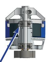
Patented motor/bearing construction with one-sided preloaded double bearing and two-part shaft for high mechanical load, smooth running and accurate grinding.
