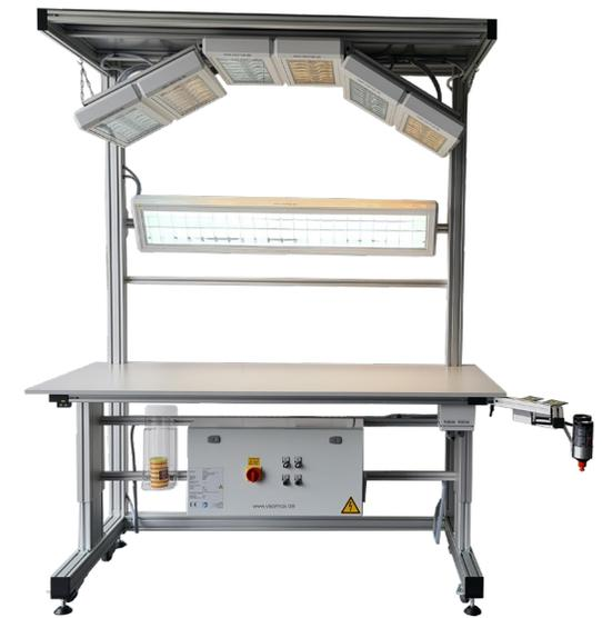
As soon as a "standard solution" doesn't apply for you, either our mobile light wall "Compact", the light wall "Compact 45°" or the "Light Wall 45°" are the ones to go for. Our light walls can be individually adapted to our client's situation and constructed accordingly. The light walls may vary in their construction, dimensions, control or in the type of lamps being used.
